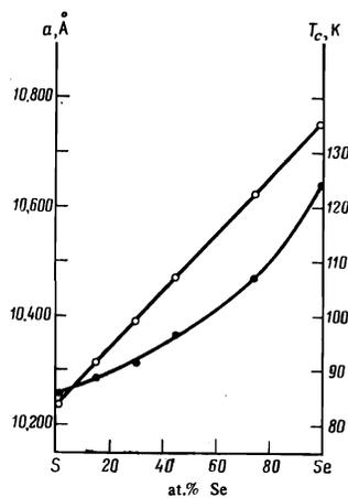
FIG. 2. Concentration dependence of lattice parameter (○) and Curie temperature (●) of solid solutions  $\text{CdCr}_2(\text{S}_x\text{Se}_{1-x})_4$ .
