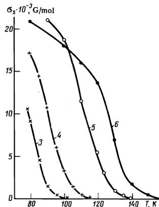
FIG. 3. Polytherms of the spontaneous magnetization of the solid-solution specimens investigated in the vicinity of their Curie points (the numbers on the curves correspond to the numbering in Table I).
