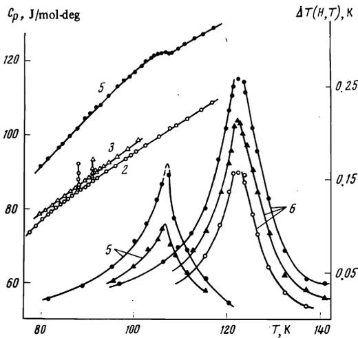
FIG. 4. Polytherms of the specific heat and of the magneto-caloric effect of the spinels: ●,  $H=2.3$  kOe; ▲,  $H=1.65$  kOe; ○,  $H=1.15$  kOe. The numbers on the curves correspond to the numbering in Table I.
