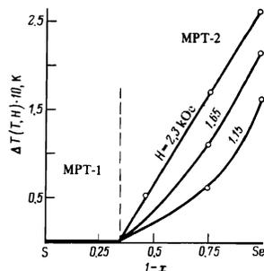
FIG. 5. Magnetoconcentration phase diagram of mutual solid solutions  $\text{CdCr}_2(\text{S}_x\text{Se}_{1-x})_4$ .
