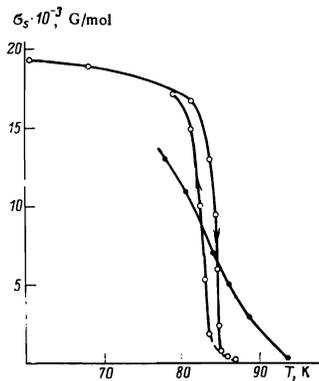
FIG. 1. Change of spontaneous magnetization of hardened (○) and annealed (●) specimens of the spinel  $\text{CdCr}_2\text{S}_4$  near the Curie point.
