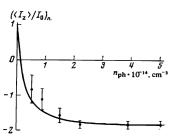
FIG. 1. Limiting dynamic polarization of the Si<sup>29</sup> nuclei  $(\langle I_{\mathfrak{a}} \rangle / I_0)_{\mathfrak{m}}$  vs photoexcited-electron concentration  $n_{ph}$  in *n*-type silicon  $(N_{\mathfrak{a}} \approx 1.7 \cdot 10^{13} \text{ cm}^{-3})$  irradiated with unpolarized light in a 4.9 kG magnetic field at 77 K. The curve was calculated with Eq. (4).
