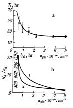
FIG. 2. a) Experimental dependence of the spin-lattice relaxation time  $T_1$  of Si<sup>29</sup> nuclei in *n*-type silicon on the concentration  $n_{ph}$  of photoexcited electrons; and b) Calculated curves showing the reciprocal degree of fillings of donor centers  $N_d/n_d$  (curve 1) and the nuclear relaxation time  $T_{1d}$  (curve 2) as functions of the photoexcited electron concentration  $n_{ph}$ .
