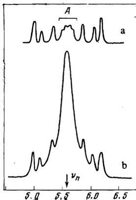
FIG. 1. Form of the ENDOR spectrum from nuclei of the third, fifth, and more distant lithium  $F$ -center coordination spheres in the absence of the Larmor ENDOR effect (Fig. a); b) the same spectrum in the presence of the Larmor ENDOR. The abscissas show the frequency of the RF field in MHz.  $H$  lies in the (001) plane and makes an angle  $28^\circ$  with the [100] axis.
