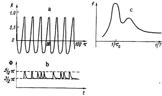
FIG. 9. Characteristics of partial stochasticity regime: a) autocorrelation function  $R(\tau)$ ; b) plot of  $\Phi(t)$ , it is seen that there is no phase accumulation; c) distribution function  $f(1/T)$ .
