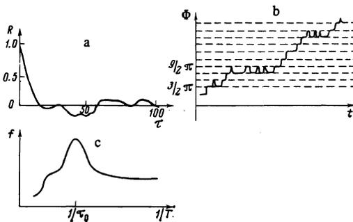
FIG. 8. Characteristics of the regime of total stochasticity: a) form of the autocorrelation function  $R(\tau)$ ; b) character of the variation of the phase difference  $\Phi$  with time, with accumulation of  $\Phi$  observed; c) distribution function in the reciprocal duration between spikes  $f(1/T)$ .
