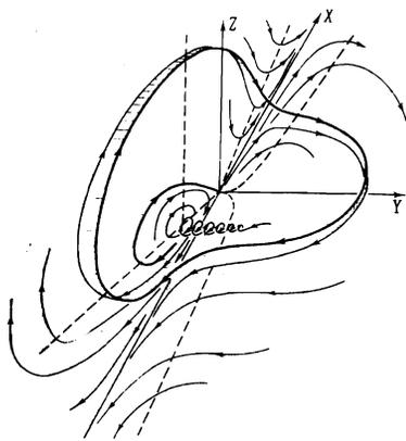
FIG. 2. Phase portrait of the system (3) in the case of exact synchronism. The equilibrium state is a saddle-node at the origin and a saddle-focus on the integral plane  $y=0$ . The steady limit cycle corresponding to a stable single-period motion is illustrated qualitatively.
