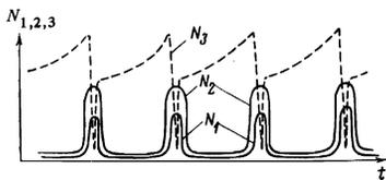
FIG. 1. Qualitative dependence of the intensity of the unstable HF mode and of the damped LF modes on the time for the steady stabilization regime.
