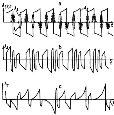
FIG. 7. The steady-state motion observed in the computer experiment: a) single-period regime at  $\delta=0$ ,  $\Delta\omega=0$ ,  $\nu\gamma>1$ ; b) multiperiodic regime at  $\delta=0$ ,  $\Delta\omega=0$ ,  $\nu\gamma\leq 1$ ; c) stochastic regime at  $\delta=0.001$  and  $\Delta\omega=0.001$ .
