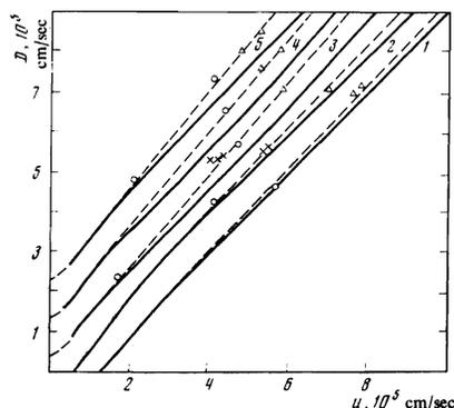
FIG. 4. Results of registration of shock adiabats of argon: 1)  $P_0 = 1$  bar, 2) 5 bar, 3) 15 bar, 4) 25 bar, 5) 50 bar. For these initial pressures, the plots are shifted in the  $D$  direction by +2, -1, 0, +1, and +2 km/sec, respectively.  $\Delta$ —<sup>[8]</sup>,  $\times$ —<sup>[5]</sup>,  $\circ$ —our data. Solid curves—calculated from <sup>[1]</sup>, dashed—calculated from (2).
