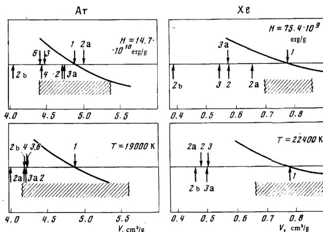
FIG. 5. Comparison of the experimental data with the theoretical models for an argon plasma ( $P_0 = 25$  bar,  $P = 9.92 \times 10^3$  bar) and a xenon plasma ( $P_0 = 50$  bar,  $P = 33.4 \times 10^3$  bar). The error corridor is shown shaded.
