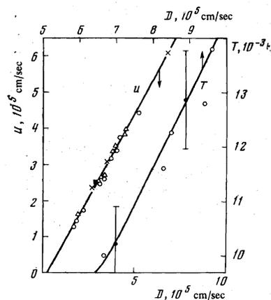
FIG. 3. Registration of the parameters of shock-compressed air. Solid curve—calculation in accordance with<sup>[16]</sup>,  $\nabla$ —<sup>[17]</sup>,  $\circ$ —<sup>[18]</sup>,  $\times$ —probe measurements,  $\blacksquare$ —optical registration (image converter). Temperature data:  $\circ$ —<sup>[11]</sup>;  $\bullet$ —our measurements.
