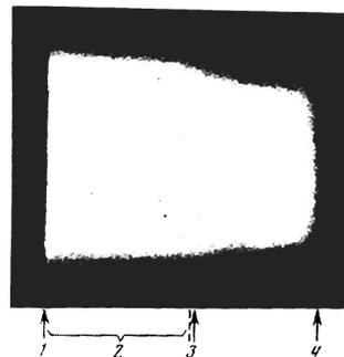
FIG. 2. Sweep of the glow of a shock-compressed plasma: lateral and rear relaxation waves.
