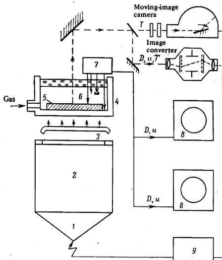
FIG. 1. Experimental setup: 1—detonation lens, 2—explosive charge, 3—metallic striker, 4—experimental assembly, 5—target, 6—investigated gas, 7—electric contact and pulse-shaping block, 8—oscilloscopes, 9—synchronization and explosion block.
