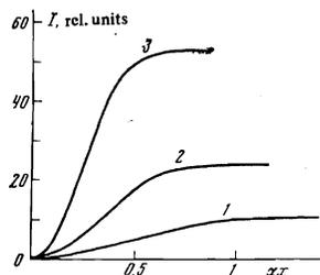
FIG. 3. The dynamics of the total sound intensity at different values of  $A$ : curve 1—for  $A = 8$ , 2—for  $A = 16$ , 3—for  $A = 32$ .
