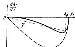
FIG. 5. Form of the phase plane of Eq. (29) with account and without account of the nonlinearity of the sound; the dashed curve is for  $\gamma = 0$ , the solid curve for  $\gamma = 14$ .
