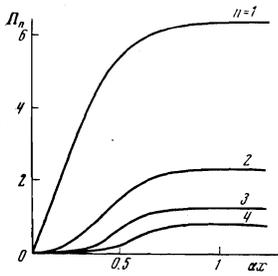
FIG. 2. Ratios of the amplitudes  $\Pi_n$  of the first several harmonics of sound at different cross sections of the medium at  $A = 16$ .
