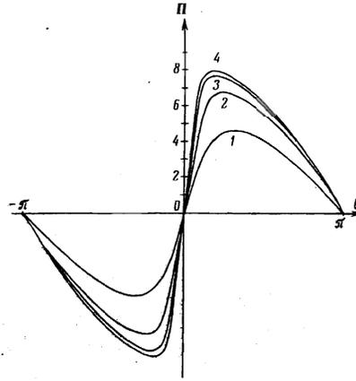
FIG. 1. Profile of the pressure wave at various distances from the boundary of the medium at  $A=20$ : curve 1—for  $\alpha x=0.3$ ; 2—for  $\alpha x=0.5$ ; 3—for  $\alpha x=0.7$ ; 4—for  $\alpha x=0.9$ .
