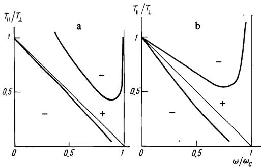
FIG. 3. The regions where  $\delta\omega$  is positive (+) and negative (-) for  $g = \omega_p^2 \bar{W}^2 / \omega_c^2 c^2 = 0.2$ ; a—in the case where the field is switched on instantaneously, b—for a packet with a smoothly increasing amplitude.
