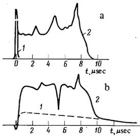
FIG. 5. Oscillograms of absorption and dispersion pulses at  $T = 1.6^\circ\text{K}$ : a—absorption, b—dispersion. Excitation intensity in relative units: 1—10, 2—20.
