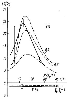
FIG. 6. Temperature dependence of the relative change in the phonon specific heat of the alloys  $V_{97.2}U_{2.8}$  and  $V_{96.5}Be_{3.5}$ , normalized to the concentration: continuous curves—experimental; dashed curves—theory with account of the change in the effective force constants.
