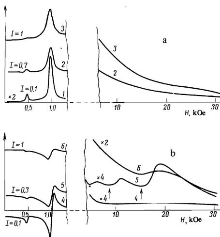
FIG. 3. Absorption (a) and dispersion (b) spectra in a magnetic field. Sample  $325 \mu$  thick.  $T = 1.8^\circ\text{K}$ . The magnetic-field direction coincides with the  $\langle 111 \rangle$  axis.
