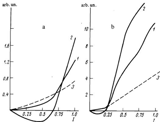
FIG. 2. Absorption and dispersion signals in a zero magnetic field at  $T = 4.2^\circ\text{K}$  (a) and  $1.45^\circ\text{K}$  (b). Curve 1—absorption, 2—dispersion, 3—absorption in a strong microwave field at a microwave power  $P_{\text{max}} \approx 10$  mW. Sample  $35 \mu$  thick.
