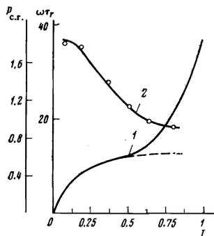
FIG. 4. Electron cyclotron resonance signal ( $M^* = 0.08 m_0$ ) vs the excitation intensity—curve 1. The abrupt growth of the signal at  $I \geq 0.6 I_{\text{max}}$  is due to suppression of the absorption, which depends little on the magnetic field. Plot of  $\omega\tau_r = 2H_c/\Delta H$  against the excitation intensity—curve 2. Sample  $325 \mu$  thick,  $T = 4.2^\circ\text{K}$ .
