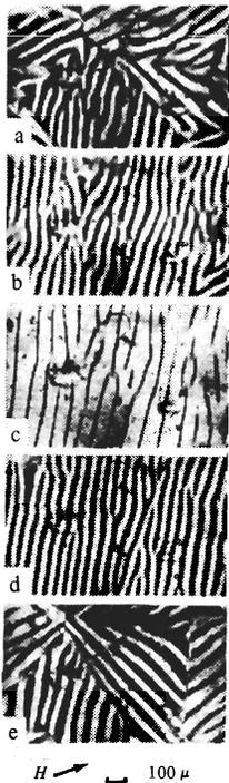
FIG. 6. Domain structure of an iron garnet crystal in various fields oriented parallel to the plane of the sample: a) 0; b) 4 Oe; c) 85 Oe; d) 0 Oe; e) -1 Oe.
