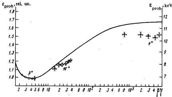
FIG. 2. Dependence of the probable ionization  $\epsilon_{\text{prob}}$  in a proportional counter on the value of  $\beta\gamma$  of the particle. Solid curve—calculation by Sternheimer's formulas.<sup>[7]</sup> Points with like symbols denote the values obtained during a single run (1–2 hours). The points for which the errors are not indicated are normalization points. The path length of the particle in the counter is 5 cm. The counter is filled with a mixture of 95% Ar + 5% CH<sub>4</sub>.
