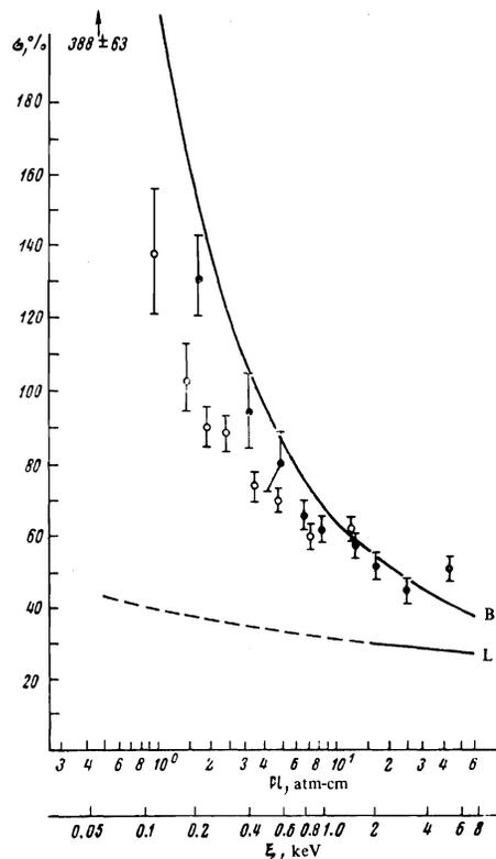
FIG. 5. Half-width  $\sigma$  of the ionization spectra of protons with momenta 2.65 GeV/sec vs. the thickness  $Pl$  of the gas layer. Smooth curves—calculation in accordance with Landau (curve L) and in accordance with Blunck and Leisegang (curve B). The counter is filled with a mixture 95% Ar + 5% CH<sub>4</sub>.  $\circ$ — $l = 5$  cm,  $\bullet$ — $l = 17$  cm.
