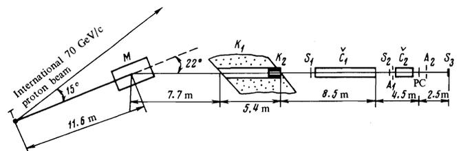
FIG. 1. Experimental setup. T—internal aluminum target of accelerator; M—analyzing magnet; K<sub>1</sub> and K<sub>2</sub>—iron collimators; S<sub>1</sub>, S<sub>2</sub>, S<sub>3</sub>—scintillation counters; A<sub>1</sub>, A<sub>2</sub>—guarding scintillation counters; PC—proportional counter;  $\check{C}_1$ ,  $\check{C}_2$ —Cerenkov counters.
