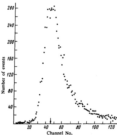
FIG. 4. Typical ionization spectrum obtained by bombarding a proportional counter with 2.65-GeV/c protons. The particle path encounter was 17 cm, the gas pressure was 1.5 atm. abs., and the gas composition 95% Ar + 5% CH<sub>4</sub>.
