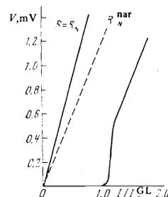
FIG. 3. Current-voltage characteristic for sample No. 11 at  $T/T_c = 0.950$ . The solid line is the CVC at  $T > T_c$ . The dashed line corresponds to the resistance of the narrow part of the film,  $R_N^{nar}$ .
