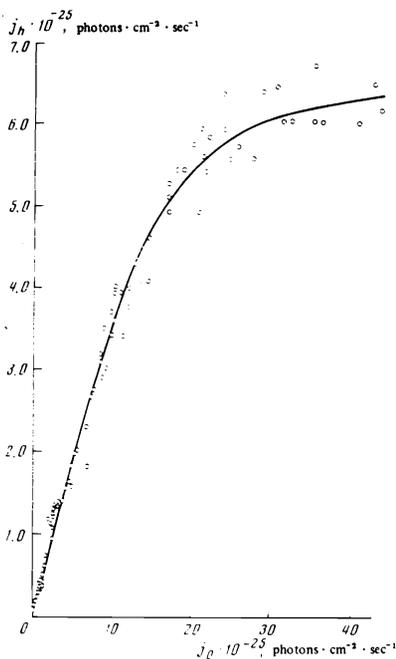
FIG. 1. Dependence of the intensity of the radiation transmitted by a sample  $j_h$  on the intensity of the radiation  $j_0$  (linear polarization) incident on  $n$ -type InAs;  $n = 8 \times 10^{16} \text{ cm}^{-3}$ ,  $\lambda = 9.5 \mu$ ,  $h = 1 \text{ mm}$ ,  $T = 300 \text{ K}$ .
