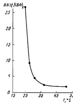
FIG. 3. Temperature dependence of the linear-circular dichroism deduced from the photoconductivity:  $j_0 = 3.3 \times 10^{25} \text{ photons} \cdot \text{cm}^{-2} \cdot \text{sec}^{-1}$ ;  $n$ -type InAs ( $n = 2.3 \times 10^{16} \text{ cm}^{-3}$ );  $\lambda = 10.6 \mu$ .
