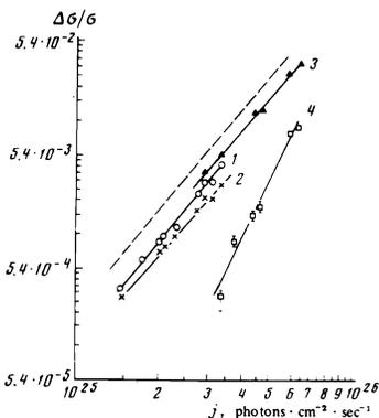
FIG. 2. Dependences of the relative photoconductivity  $\Delta\sigma/\sigma$  on the intensity  $j_0$  of light incident on  $n$ -type InAs ( $n = 2.3 \times 10^{16} \text{ cm}^{-3}$ ): 1), 2)  $\lambda = 9.5 \mu$ ; 3), 4)  $\lambda = 10.6 \mu$ ; 1), 3) linear polarization; 2), 4) circular polarization;  $T = 300 \text{ K}$ . The dashed line represents the dependence  $\Delta\sigma/\sigma \propto j_0^3$ .
