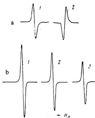
FIG. 1. Signals representing the variation in the electrical conductivity of a plasma: (a) magnetic resonance in the ground  $5^2S_{1/2}$  state of  $\text{Rb}^{85}$  atoms ( $f_0 = 290$  kHz); (b) magnetic resonance in the metastable  $2^3S_1$  state of  $\text{He}^4$  ( $f_0 = 1760$  kHz).
