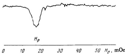
FIG. 3. Signal showing the variation in the electrical conductivity of plasma for the difference frequency  $\Delta f = f_0(\text{He}^*) - f_0(\text{Rb}^{85})$  in the case of simultaneous magnetic resonance of the  $\text{Rb}^{85}$  and  $\text{He}^*$  atoms [ $f_0(\text{He}^*) = 48.4$  kHz,  $f_0(\text{Rb}^{85}) = 8.1$  kHz].
