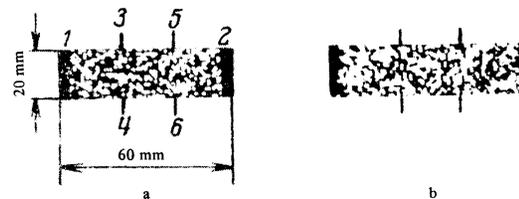
FIG. 1. a) Two-dimensional samples in which 390 holes have been punched; 1, 2—current contacts, 3, 4 and 5, 6—two pairs of Hall contacts; b) photograph of one of the fifteen planar layers composing the three-dimensional sample ( $x = 0.6$ ).
