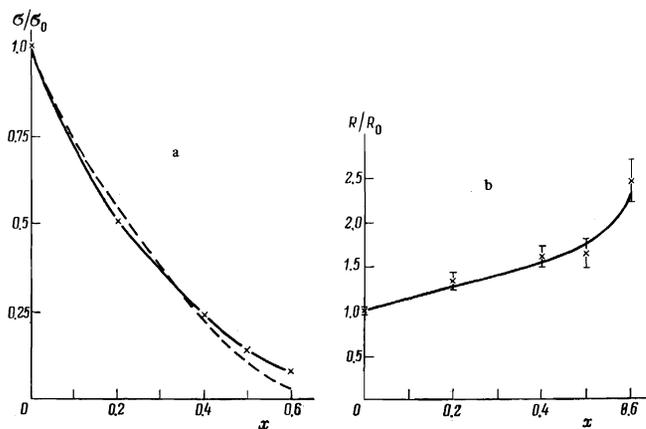
FIG. 4. Dependence of the relative conductivity (Fig. a) and relative Hall constant (Fig. b) on  $x$ . The dashed line shows  $\sigma/\sigma_0$  from the data of [1].
