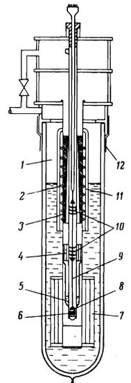
FIG. 1. Scheme of apparatus: 1—helium bath, 2—heater, 3—carbon "pump," 4—condenser, 5—liquid  $He^3$ , 6—sample, 7—solenoid, 8—carbon thermometer, 9—insert, 10—radiation screen, 11—vacuum "jacket," 12—rubber sleeve.
