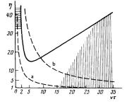
FIG. 3. Regions of unstable laser action, nutational oscillations, and oscillations accompanied by full modulation of the field. The hyperbolas a and b correspond to A = 50 and A = 300.
