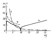
FIG. 4. Oscillation frequency  $\omega_1$ , supernutation frequency  $D\sqrt{2R_s}$ , and reciprocal of the photon lifetime in a resonator  $\nu$ plotted as a function of  $\sqrt{\eta}$  for A = 10<sup>3</sup>: a)  $\omega_1 \tau$ ; b)  $D\tau \sqrt{2R_s}$ ; c) ντ.
