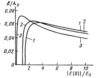
FIG. 3. Dependence of the penetration depth of the field into the plasma on the electric-field intensity for  $m=1$ : 1)  $\gamma=1$ ; 2)  $\gamma=1.2$ ; 3)  $\gamma=1.9$ .
