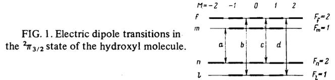
FIG. 1. Electric dipole transitions in the  $^2\Pi_{3/2}$  state of the hydroxyl molecule.
