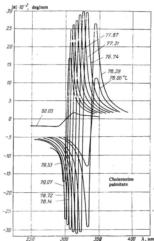
FIG. 1. Dispersion of the optical activity of palmitate.
