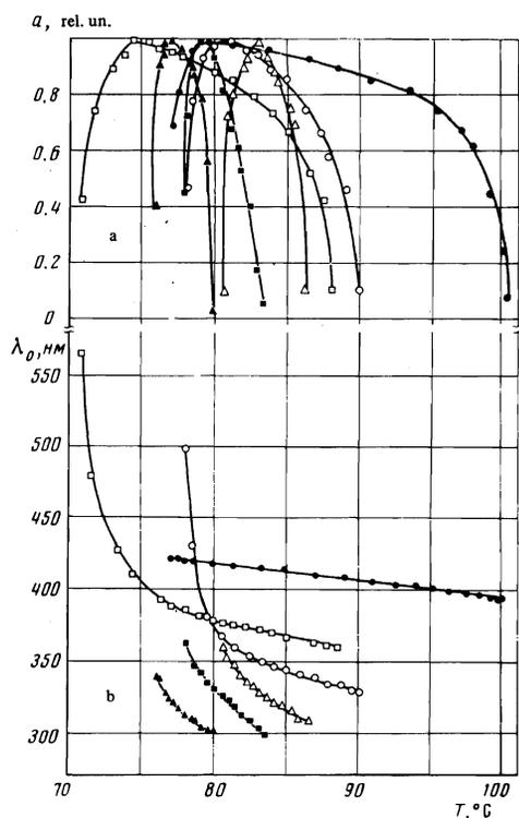
FIG. 3. Temperature dependence of the amplitude  $[\alpha]$  in relative units (a) and of the wavelength of the inversion point of the curve  $[\alpha]$  (b) for valerate ( $\bullet$ ),  $a_{\max} = 3468^\circ$ ; palmitate ( $\blacktriangle$ ),  $a_{\max} = 6089^\circ$ ; laurate ( $\Delta$ ),  $a_{\max} = 5438^\circ$ ; myristate ( $\blacksquare$ ),  $a_{\max} = 4815^\circ$ ; caprylate ( $\circ$ ),  $a_{\max} = 3882^\circ$ ; pelargonate ( $\square$ ),  $a_{\max} = 2623^\circ$ .
