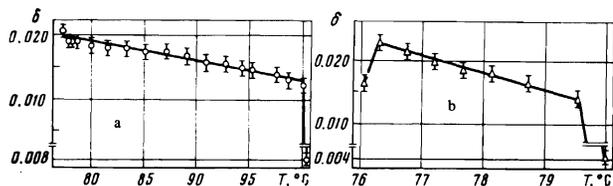
FIG. 4. Variation of the anisotropy parameter of the planar structure of valerate (a) and palmitate (b) in the region of the cholesteric-mesophase temperatures.
