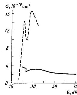
FIG. 1. Cross section for the excitation of the  $4p^2D_{5/2}$  level: solid line—calculation, dashed—experiment [23,24].
