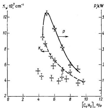
FIG. 3. Dependence of the maximum gain  $K_\nu$  ( $\Delta$ —present work,  $\circ$ —[18]) and of the laser-radiation power  $P$  on the  $C_2H_2$  concentration in the initial mixture.
