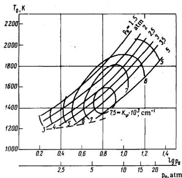
FIG. 4. Dependence of the beam  $K_\nu$  on the running values of the stagnation parameters (pressure  $p_0$ , temperature  $T_0$ ) for different initial values  $p_{in}$  of the initial 5.5% acetylene-air mixture. The change of the stagnation parameters below the dashed line was hindered by the appearance of a shock wave in the resonator cavity.
