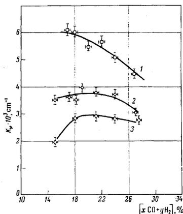
FIG. 7. Dependence of the maximum values of the gain  $K_{\nu}$  for model mixtures: curve 1—for  $2\text{CO} + \text{H}_2$ , 2— $3\text{CO} + 4\text{H}_2$ , 3— $\text{CO} + 2\text{H}_2$ .
