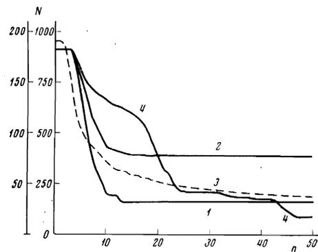
FIG. 4. Drop in current with number of turns in perturbed case (curve 1— $\varphi_S = 0.10$ , 2— $\varphi_S = 0.15$ , 3— $\varphi_S = 0.32$ ) and under the influence of a slow perturbation (4— $\varphi_S = 0.15$ ). The right-hand scale of  $N$  is given only for curve 3.
