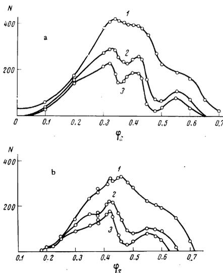
FIG. 2. Current-voltage characteristics of a microtron: a— $L = 0$ , for curves 1, 2, and 3  $n$  is respectively 8, 15, and 28; b— $L = 1.45 c/\omega$ , for curves 1, 2, and 3  $n$  is respectively 8, 15, and 25.
