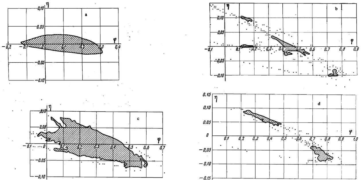
FIG. 3. Phase-stability region calculated for 30 turns: a— $\varphi_S = 0.15$ , b— $\varphi_S = 0.30$ , c— $\varphi_S = 0.445$ , d— $\varphi_S = 0.594$ .
