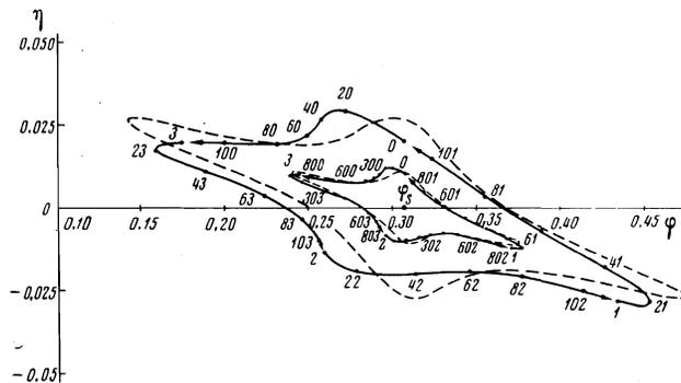
FIG. 1. Phase trajectories for  $\nu = \pi/2$  ( $\varphi_s = 0.308$ ,  $\varphi = \varphi_s + \psi$ ). Solid curves—numerical calculation by computer, dashed curves—plotted from Eq. (5) and drawn through points No. 80 (outer curve) and No. 600.
