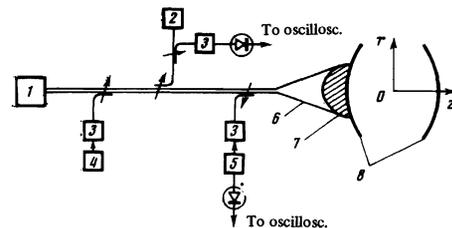
FIG. 1. Diagram of setup: 1—magnetron, 2—VI-1 power meter, 3—attenuator, 4—klystron oscillator, 5—flow-through resonator, 6—horn, 7—teflon lens, 8—open resonator.
