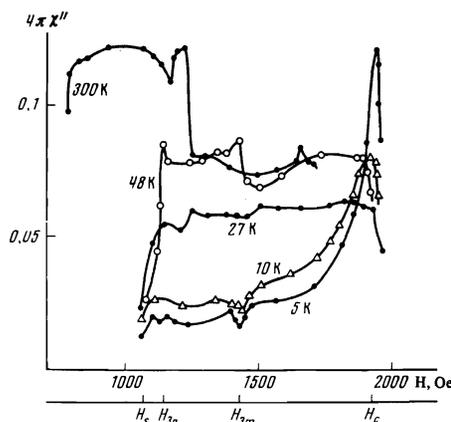
FIG. 2. Same as in Fig. 1, for magnetization of the ferrite along the hard axis  $[100]$ . The values of the fields  $H_S$ ,  $H_{3p}$ ,  $H_{3m}$ , and  $H_C$  on the horizontal axis correspond to specimen temperature 5 K.
