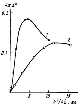
FIG. 3. Dependence of the imaginary part of the nonlinear susceptibility on the excess of the pumping field over the threshold level, for two values of the constant magnetic field:  $H = H_C$  (curve 1) and  $H = H_{3m}$  (curve 2). Specimen, a YIG sphere of diameter 2.25 mm. Specimen temperature 5 K.
