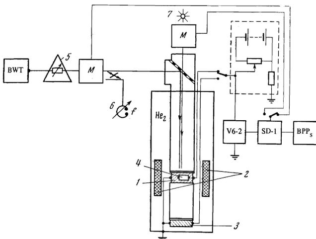
FIG. 1. Block diagram of the experimental apparatus: 1—investigated sample; 2—superconducting solenoid; 3—radiation detector; 4—carbon thermometer; 5—attenuator; 6—frequency meter; 7—illumination source; M—modulator, BWT—backward-wave tube; V6-2—low-frequency amplifier; SD-1—synchronous detector, BPP<sub>s</sub>—recording instrument.
