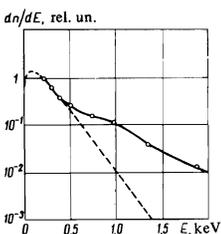
FIG. 1. Plasma-ion energy spectrum at the start of the decay. The cold part is extrapolated by a Maxwellian distribution with  $T = 150$  eV.
