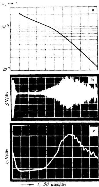
FIG. 2. Plasma decay process: a—variation of density, b—RF-noise signal; c—floating-potential signal.
