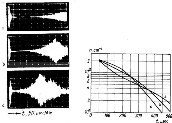
FIG. 5. Development of plasma instability at different initial ion temperatures: a— $T_i \approx 50$  eV, ordinate scale 0.5 V/div; b— $T_i \approx 100$  eV, scale 2.0 V/div; c— $T_i \approx 150$  eV, scale 5.0 V/div.
