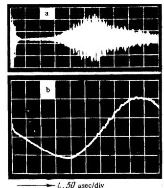
FIG. 4. Production of hot ions under the influence of instability: a—RF-noise signal, b—signal of neutral atoms with  $E = 2 \text{ keV}$ .
