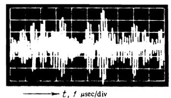
FIG. 3. “Microstructure” of unstable oscillations.
