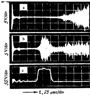
FIG. 8. Excitation of instability by artificially raising the plasma potential: a—RF-noise signal in ordinary decay; b—the same when a potential pulse (100 V) is applied, c—applied potential pulse.
