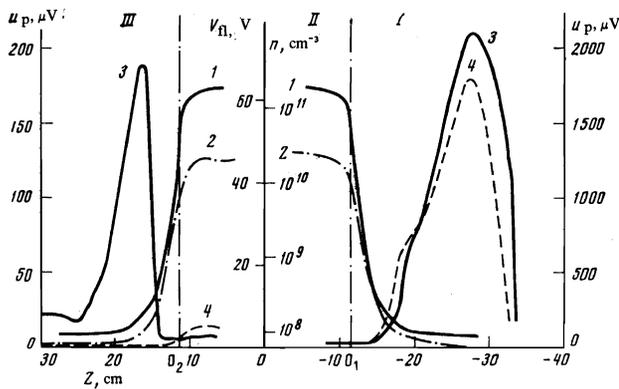
FIG. 2. Axial distribution of the plasma density (1), floating-probe potential (2), and amplitude of hf oscillations (3, 4);  $f = 19$  MHz.
