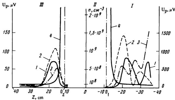
FIG. 4. Axial distributions of the amplitude of hf oscillations (1-3) and plasma density (4).  $Z_e = -34$  cm; 1- $f = 19$  MHz; 2- $f = 24$  MHz; 3- $f = 32$  MHz.
