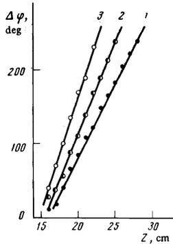
FIG. 5. Axial variation in the phase change in region III: 1- $f = 19$  MHz; 2- $f = 24$  MHz; 3- $f = 32$  MHz.
