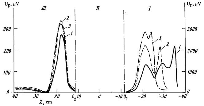
FIG. 3. Axial distributions of the amplitude of hf oscillations; 1 –  $Z_e = -35$  cm; 2 –  $Z_e = -28$  cm; 3 –  $Z_e = -24$  cm;  $f = 28$  MHz.
