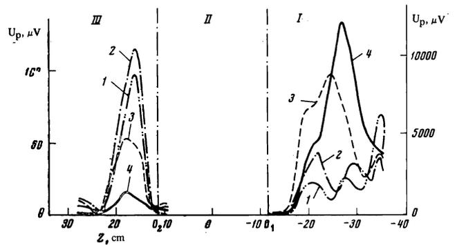
FIG. 6. Axial distributions of the amplitude of hf oscillations: 1- $I_a = 0.3$  A,  $n = 9.7 \times 10^7$  cm<sup>-3</sup>; 2- $I_a = 0.4$  A,  $n = 1.3 \times 10^8$  cm<sup>-3</sup>; 3- $I_a = 0.8$  A,  $n = 2.1 \times 10^8$  cm<sup>-3</sup>; 4- $I_a = 1$  A,  $n = 2.9 \times 10^8$  cm<sup>-3</sup>;  $Z_e = -34$  cm;  $f = 28$  MHz.
