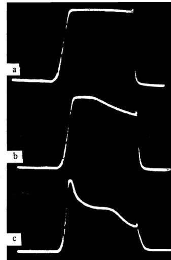
FIG. 3. Photographs of pulses reflected from the resonator at different values of the microwave magnetic field  $h$ : a)  $h < h_c^{(1)}$ , b)  $h_c^{(1)} < h < h_c^{(2)}$ , c)  $h_c^{(2)} < h < h_c^{(3)}$ .
