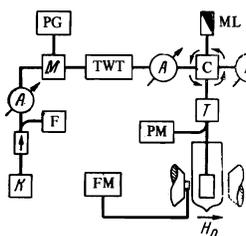
FIG. 2. Block diagram of spectrometer: A—attenuator, PG—pulse generator, D—detector, PM—power meter, FM—magnetic-field meter, K—klystron, TWT—traveling wave tube, M—microwave-power modulator, O—oscilloscope, ML—matched load, T—impedance transformer, C—circulator, F—frequency meter.
