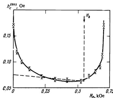
FIG. 9. Field dependence of the threshold amplitude of parallel pumping at the frequency  $\omega_p = 2\pi \times 875$  MHz ( $T = 1.7^\circ$  K). The dashed line is drawn in accordance with the formula (18c) with  $Q_{1nk} = \text{const}$ ; the boundary field  $H_b$  was calculated from the condition  $\omega_p = 2\Omega_{1nk}$ . At  $H_0 > H_b$ , a 3–3 process with  $k \lesssim k_c^{(np)}$  is possible, see Fig. 1.
