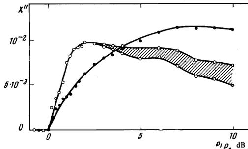
FIG. 10. Behavior of the beyond-threshold susceptibility  $\chi''$ : ●—for en processes, ○—for ep process;  $T = 1.7^\circ$  K,  $H_0 = 500$  Oe.
