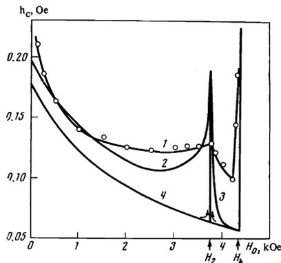
FIG. 13. For use in comparison of theory with experiment at 35 GHz. Curve 1 was plotted from the experimental data of<sup>[17a]</sup>. Curves 2 and 3 are plots of formulas (22a) and (22b) with the parameters given in the text (Sec. 4A). Curve 4 corresponds to the case when there is no magnon-phonon coupling ( $\omega_{\text{med}} = 0$ ).
