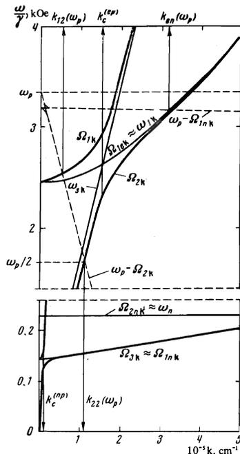
FIG. 1. Spectrum of  $\text{MnCO}_3$  at  $H_0 = 0.5$  kOe,  $T = 1.7^\circ \text{K}$ ,  $H_D = 4.4$  kOe,  $\omega_E \omega_N / \gamma^2 = 5.8 \text{ T}^{-1} \text{ kOe}$ ,  $\omega_E \omega_{mes} / \gamma^2 = 0.3 \text{ kOe}^2$ ,  $\omega_E \omega_{med} / \gamma^2 = 0.4 \text{ kOe}^2$ ,  $v_m = 1.07 \times 10^5 \text{ cm/sec}$ ,  $v_s = 3.0 \times 10^5 \text{ cm/sec}$ . Pump frequency  $\omega_p / \gamma = 3.3 \text{ kOe}$ .
