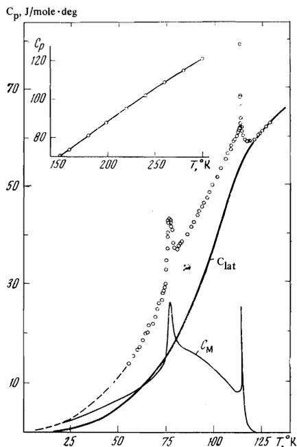
FIG. 3. Temperature dependence of heat capacity of  $\text{YVO}_3$ .
