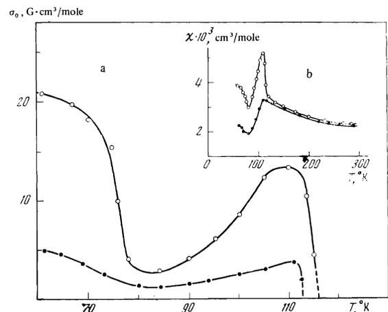
FIG. 1. a) Temperature dependence of the spontaneous ferromagnetic moment of  $YVO_3$ ; b) polytherms of the magnetic susceptibility for a sample annealed at  $T = 1300^\circ\text{C}$  (○) and for a non-annealed sample (●).
