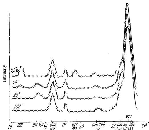
FIG. 2. Neutron diffraction patterns of  $\text{YVO}_3$ .
