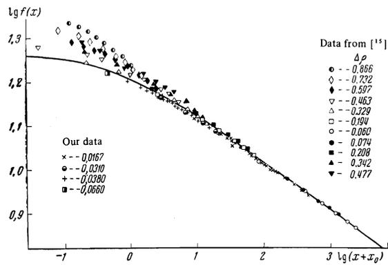
FIG. 5. Scaling function of the specific heat in the "zeroth-order approximation" from Eq. (2), with the temperature dependence of  $B(T)$  and  $\mu''(\rho_C, T)$  taken into account. The solid line is the same as in Fig. 3.
