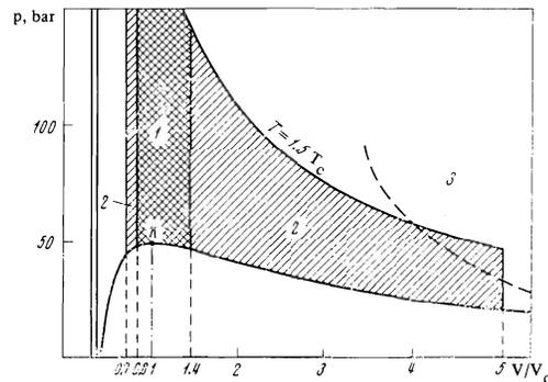
FIG. 1. P-V diagram of Ar. Area 1 corresponds to the region of validity of the "zeroth-order approximation" given by Eqs. (1) and (2), and area 2 to the introduction of the first correction ( $\sim \Delta \rho^2$ ) to Eq. (2). The dashed line is the tentative boundary of the region 3 in which the virial equation of state, with second and third virial coefficients<sup>[14-16]</sup>, is valid.
