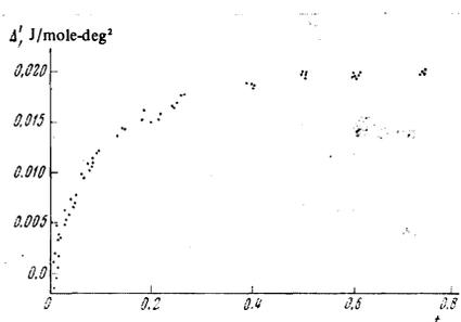
FIG. 9. Difference  $\Delta' = C_V^{\text{exp}}/T - (At^{-\alpha} + B)$  between the experimental specific heat  $C_V$  of Ar on the critical isochore at  $T > T_C$  and the values given by the asymptotic law (13).
