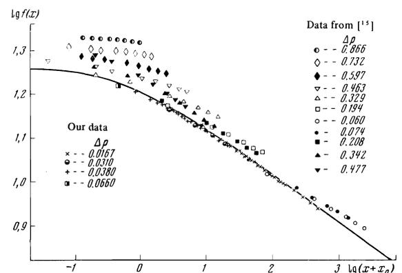
FIG. 3. Scaling function of the specific heat from Eq. (2) in the approximation  $\mu''(\rho_C, T) = \text{const}$  and  $B(T) = \text{const}$ . The solid line is plotted from the LM equation (10) with the parameters (17).
