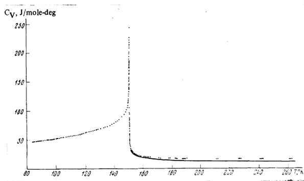
FIG. 8. Temperature dependence of the specific heat  $C_V$  on the critical isochore over a wide temperature interval. The solid line corresponds to the asymptotic law (13).
