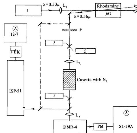
FIG. 3. Block diagram of the experimental setup used to investigate SRS excitation in liquid nitrogen by optical noise: 1) pump generator, 2) calorimeters, ISP-51) spectrograph, FEK) coaxial photocell, DMR-4) double monochromator, I2-7 and S1-19A) oscillographs,  $L_{1,2,3}$ ) lenses.
