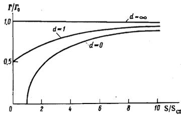
FIG. 2. The dependence of the increment of the noise-pump excited SRS on the reduced spectral density of the pump. The curve parameter  $d = \Delta\nu_0/\Delta\nu_p$  is the ratio of the spontaneous Raman line width to the spectral width of the pump.
