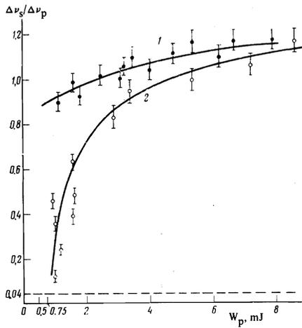
FIG. 6. The relative spectral line width of the first Stokes component excited by the noise pump as a function of the pump energy. The curve 1 corresponds to the case when  $L \approx L_{\text{coh}}$ , the curve 2 to the case when  $L \gg L_{\text{coh}}$ . The dashed line indicates the theoretical value of the minimum band width of the Stokes wave for  $L \gg L_{\text{coh}}$ .
