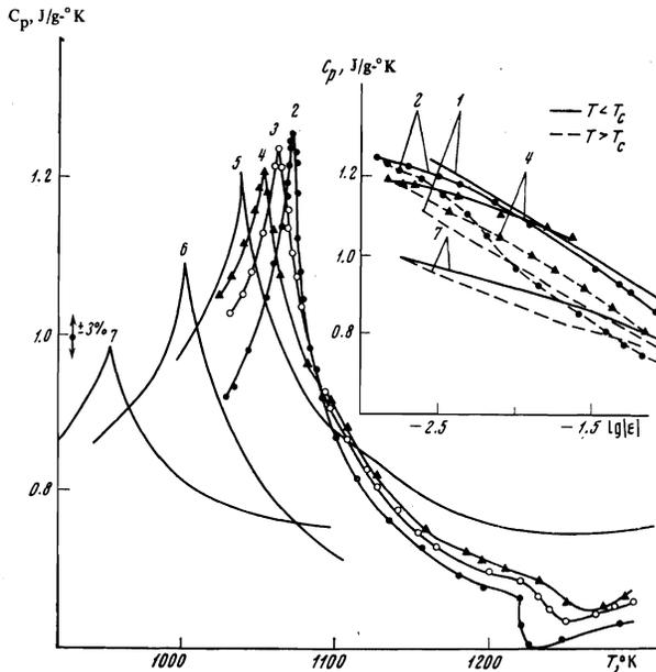
FIG. 3. Specific heat of Fe and of solid solutions of Si in Fe in the region of the Curie point. Curves: 1) average data of [6,7] for Fe; 3, 4) our data for alloys of Fe with 0.8 and 1.77 at.% Si; 5) data of [16] for Fe with 3.34 at.% Si; 6, 7) data of [17] for Fe with 5.89 and 10.83 at.% Si.
