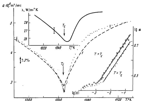
FIG. 1. Temperature diffusivity  $a$  and thermal conductivity  $\lambda$  of iron in the region of the Curie point. Curve 1—data of [8].
