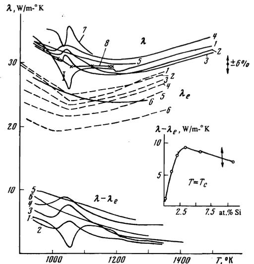
FIG. 4. Total thermal conductivity  $\lambda$ , its electronic component  $\lambda_e$ , and its "lattice" component  $\lambda - \lambda_e$  in solid solutions of Si and Fe at high temperatures. Curves 1-6) Fe and 0.0, 0.80, 1.77, 3.00, 5.79, and 11.15 at.% Si, respectively; 7) data of [5]; 8) data of [2]. The insert shows  $\lambda - \lambda_e$  at  $T = T_c$  as a function of the silicon content.
