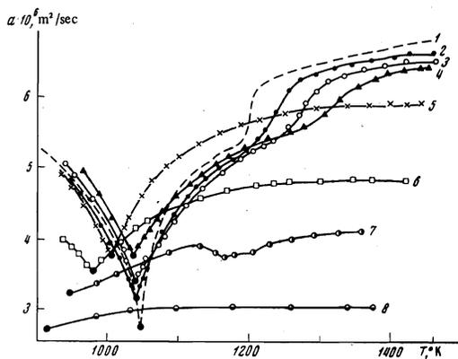
FIG. 2. Diffusivity of solid solutions of Si in Fe at high temperatures. Curves 1-8—values for Fe alloys with 0.0, 0.80, 1.77, 3.00, 5.79, 11.15, 18.11, and 25.0 at.% Si, respectively. The dark large symbols distinguish the diffusivity values at the minimum.
