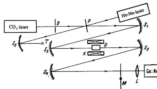
FIG. 1. Experimental setup: D—diaphragm, P—BaF<sub>2</sub> beam-splitting plate, S<sub>1-5</sub>—mirrors, K—solenoid, O—sample, T—thermocouple, M—mechanical chopper, and L—field lens.
