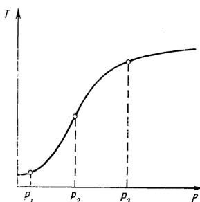
FIG. 3. Transmission  $T$  of the nitrobenzene solution of dye No. 3955 as a function of the power  $P$  of the neodymium laser radiation.
