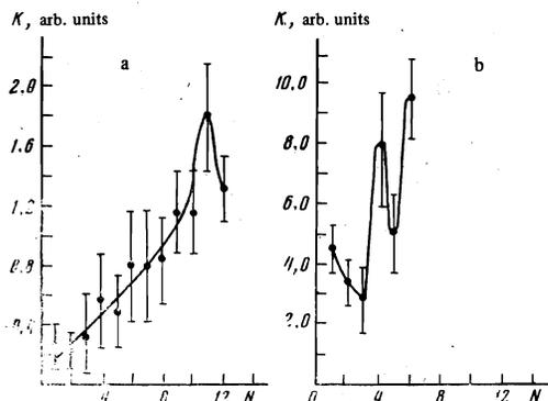
FIG. 6. Measured transformation coefficient  $K$  as a function of the number  $N$  of USP transits in the STM. The output power in case b is higher by an order of magnitude than in case a.
