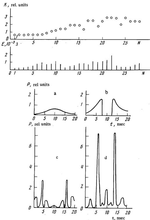
FIG. 7. Calculated change in the USP energy  $E$ , transformation coefficient  $K$ , and USP shape (a-e) as functions of the number  $N$  of passes through the STM; a - USP shape after fifth pass, b - after eighth pass, c - after eleventh pass, d - after twenty-first pass.
