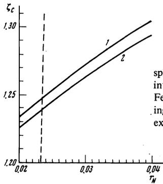
FIG. 3. The critical charge for a spherical nucleus with screening taken into account according to the Thomas-Fermi model (curve 1) and the screening (curve 2) (the nuclear radius  $r_N$  is expressed in units of  $\hbar/m_e c = 386$  F).
