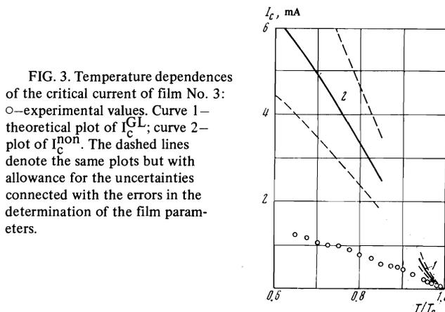
FIG. 3. Temperature dependences of the critical current of film No. 3:  $\circ$ —experimental values. Curve 1— $I_C^{GL}$ ; curve 2— $I_C^{non}$ . The dashed lines denote the same plots but with allowance for the uncertainties connected with the errors in the determination of the film parameters.
