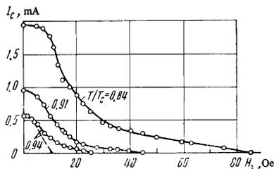
FIG. 4. Plot of  $I_c(H_{\perp})$  for film No. 1. Dashed line—theoretical plot of formula (10).
