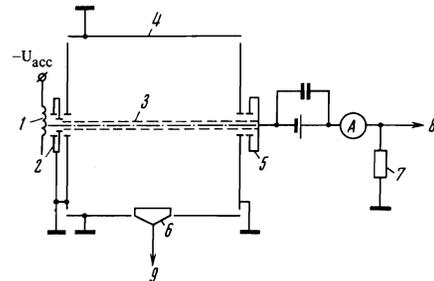
FIG. 1. Diagram of the apparatus: 1—cathode, 2—diaphragm, 3—beam, 4—equipotential region, 5—anode, 6—probe, 7—resistor, 8—to the spectrum analyzer, 9—to the electrometer amplifier.
