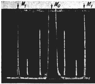
FIG. 2. Spectrum of the electron-ion oscillations in the anode current. Argon,  $p \approx 6 \times 10^{-6}$  mm Hg,  $U_{acc} = 150$  V,  $U_a = 15$  V,  $I = 350$   $\mu$ A.  $M_0$  and  $M_1$  are frequency markers indicating frequencies of 0 and 700 kHz, respectively.
