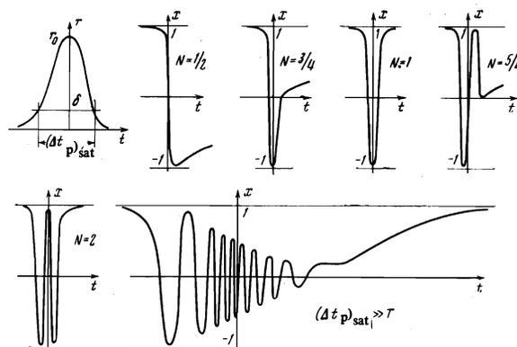
FIG. 2. Relaxation of the population in the field of a short pulse ( $\Delta t_{\text{min}} \ll 1/\delta$ ).
