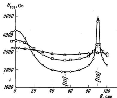
FIG. 1. Dependences of the resonance field of  $\text{Y}_{3-x}\text{Nd}_x\text{Fe}_5\text{O}_{12}$  single crystals on the angle between the direction of the saturation magnetization and the [100] axis in the (110) plane. Frequency  $f = 8.360$  GHz;  $T = 4.2^\circ\text{K}$ ;  $\Delta$ - $x = 0.0$ ;  $\square$ - $x = 0.006$ ;  $\circ$ - $x = 0.015$ .
