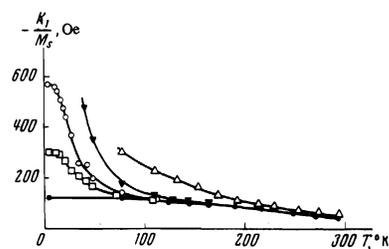
FIG. 2. Temperature dependences of  $K_1/M_S$  for  $\text{Y}_{3-x}\text{Nd}_x\text{Fe}_5\text{O}_{12}$  single crystals:  $\bullet$ - $x = 0.00$ ;  $\square$ - $x = 0.006$ ;  $\circ$ - $x = 0.015$ ;  $\blacktriangledown$ - $x = 0.03$ ;  $\Delta$ - $x = 0.09$ .
