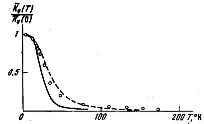
FIG. 4. Temperature dependences of  $\bar{K}_4(T)/\bar{K}_4(0)$ : the points represent the experimental values and the continuous and dashed curves correspond to the one-ion and two-ion models.
