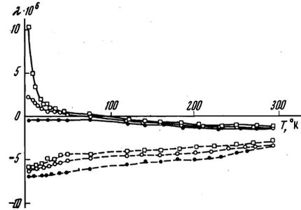
FIG. 5. Temperature dependences of the magnetostriction constants  $\lambda_{100}$  and  $\lambda_{111}$  of  $Y_{3-x}Nd_xFe_5O_{12}$  single crystals:  $\bullet$ — $x = 0.0$ ;  $\circ$ — $x = 0.006$ ;  $\square$ — $x = 0.015$ ; the dashed curves represent  $\lambda_{111}$  and the continuous curves  $\lambda_{100}$ .
