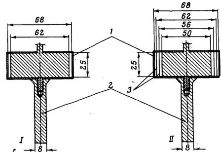
FIG. 1. Schematic diagram of the apparatus: I—with a single ring gap; II—with three coaxial ring gaps (the dimensions are in millimeters).
