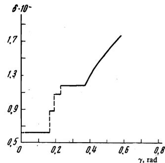
FIG. 2. Amplitude dependence of the logarithmic damping decrement of the oscillations for apparatus II.
