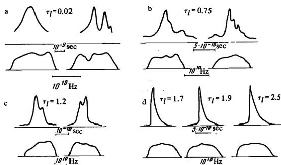
FIG. 6. Intensity diagrams for pulses and the corresponding spectra for various  $\tau_l$  (in  $\mu\text{sec}$ ).
