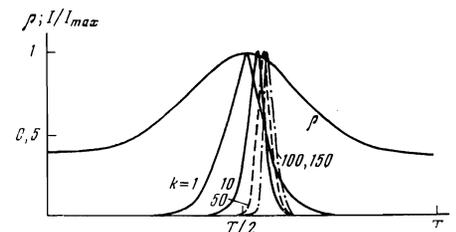
FIG. 1. Modulator transmission  $\rho(t)$  per period and pulse envelope family for different round-trip numbers  $k$ .
