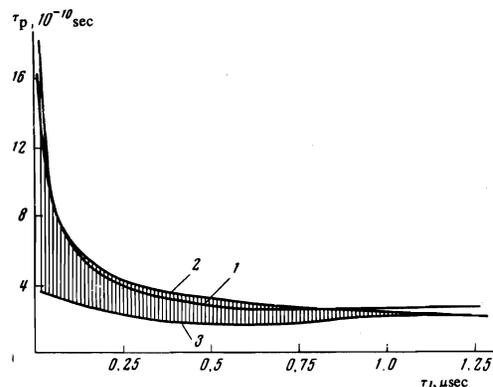
FIG. 7. Pulse length as a function of linear development time; line 1 — theoretical; lines 2 and 3 limit the region of experimental data.
