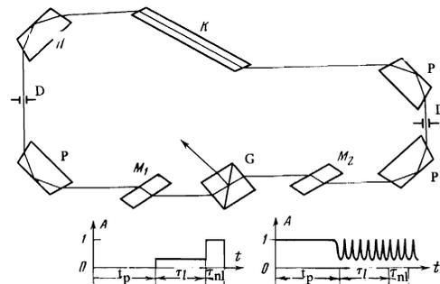
FIG. 5. Experimental setup:  $K$  - crystal;  $P$  - nondispersion prisms;  $D$  - iris;  $M_1, M_2$  - modulators;  $G$  - Glan prism. Bottom: nomograms illustrating the transmission of electro-optical modulators:  $t_p$  - pumping time;  $\tau_l$  - linear amplification time;  $\tau_{nl}$  - nonlinear amplification time.
