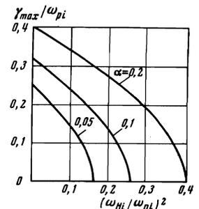
FIG. 1. Maximum growth rate of oscillations as a function of the magnetic field,  $\alpha = n_b/N_i$ .
