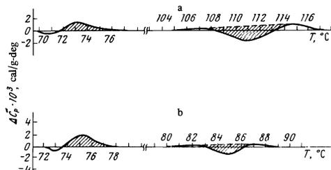
FIG. 4. The same as in Fig. 3, for the alloy In + 20.0 at.% Tl: a — unaged bulky sample, b — freshly extruded wire sample. The left and right halves of each figure pertain to the fcc  $\rightarrow$  fct and fct  $\rightarrow$  fcc transitions, respectively. The areas corresponding to the latent heat are shown shaded.
