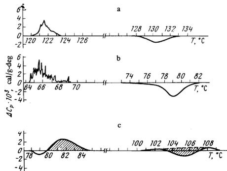
FIG. 3. Anomalies of the specific heat of In + 4.85 at.% Cd alloy in the region of the fct  $\rightleftharpoons$  fcc transitions, registered with an automatic microcalorimeter: a — bulky aged sample, b — aged wire sample, c — freshly extruded wire sample (the shaded area corresponds to the latent heat). The left and right halves of each figure correspond to fcc  $\rightarrow$  fct and fct  $\rightarrow$  fcc transitions, respectively.
