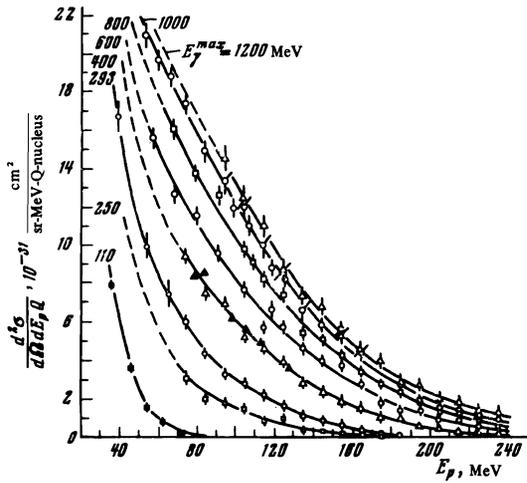
FIG. 1. Energy spectra of photoprotons from  $C^{12}$  at an angle  $\theta_{\text{lab}} = 90^\circ$  for bremsstrahlung photons with maximum energy from 110 to 1200 MeV. The errors are statistical. Hollow points—results of the present work, solid points—data from other sources: ■—ref. 12, ●—ref. 4, ▲—ref. 5.
