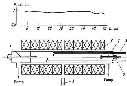
FIG. 1. Schematic diagram of the apparatus: 1—electron gun, 2—collector, 3—movable coaxial microwave probe, 4—movable double probe, 5—magnetic field coils, 6—photomultiplier with NaI(Tl) crystal. The distribution of the homogeneous magnetic field along the axis is shown above.
