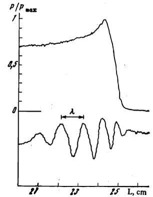
FIG. 7. Distribution of the oscillation intensity along the system and variation of the wavelength at  $f = 2000$  MHz. The beam energy  $U_b = 1.3$  keV.
