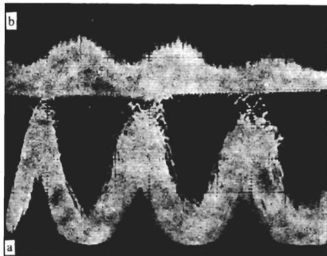
FIG. 10. Oscillations of the ion saturation current (a) and the intensities of the x-ray emission from the plasma (b); sweep time  $t = 10 \mu\text{sec/cm}$ .
