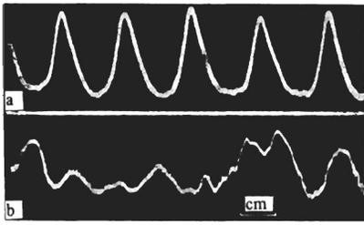
FIG. 3. Oscillograms of the ion saturation current from the probe under conditions of regular and irregular oscillations. The sweep time is  $\tau = 10 \mu\text{sec/cm}$  for oscillogram a and  $\tau = 50 \mu\text{sec}$  for oscillogram b.
