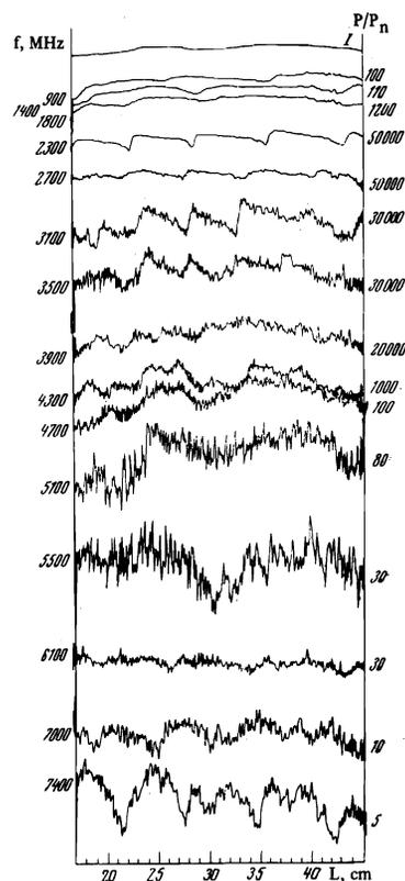
FIG. 2. The distribution of oscillation intensity along the axis of the system in homogeneous magnetic field ( $f$  is the frequency of the received oscillations,  $P/P_n$  is the ratio of the power of the received oscillations to the noise power; the frequency in MHz is on the left). Curve 1 is the ion saturation current.  $H = 2200$  Oe, the beam current is  $I_b = 70$  the beam energy is  $U_b = 1$  keV, the pressure in  $p = 3 \times 10^{-5}$  mm Hg,  $n_{\min}/n_{\max} = 10^{-1}$ .
