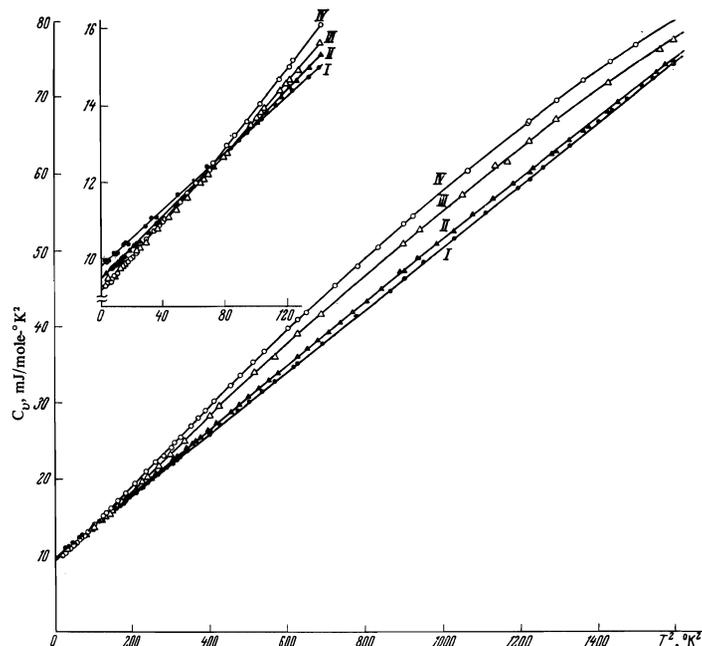
FIG. 1. Specific heat of V and of its alloys with Ta (I—V; II— $V_{99.18}\text{Ta}_{0.82}$ ; III— $V_{96.45}\text{Ta}_{3.55}$ ; IV— $V_{94.32}\text{Ta}_{5.68}$ ) in the normal state.
