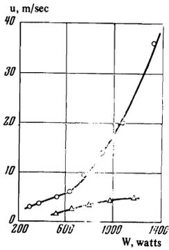
FIG. 5. Velocity of uhf discharge versus generated power level in tubes of different diameters at  $P = 22$  Torr:  $\circ$ — $\phi$  20 mm,  $\Delta$ — $\phi$  6.5 mm.
