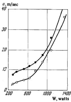
FIG. 1. Velocity of uhf discharge versus level of generated power in a tube of 20-mm diameter: ●—P = 16 Torr, ○—P = 22 Torr.
