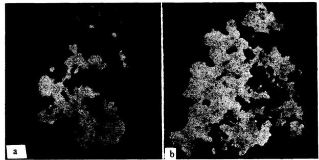
FIG. 2. Broadening of ion field emission image of bombarded tungsten microcrystal: a—microgram taken immediately after bombardment, b—after deformation at  $\sigma \approx 500$  kgf/mm<sup>2</sup>.
