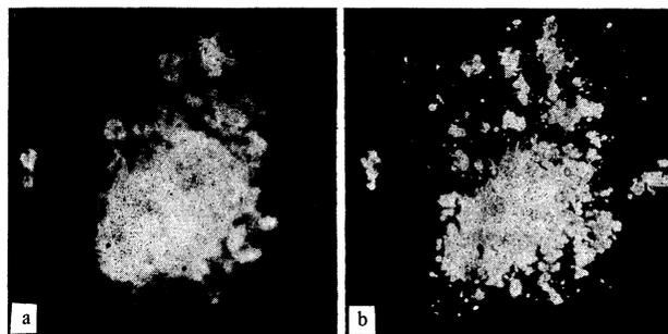
FIG. 4. Electron (a) and ion (b) field emission pictures of a crystal bombarded at 21°K.
