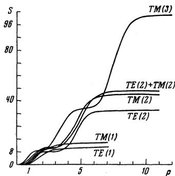
FIG. 5. Distribution of energy flux in the cross section of self-focusing cylindrical waveguides: TE(1); TE(2)—ground and first excited states of one-component waveguide; TM(1), TM(2), TM(3)—ground and first two excited states of two-component waveguide; TE(2) + TM(2)—three-component waveguide state found.
