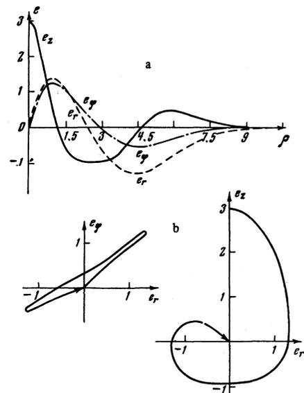
FIG. 4. a—Distribution of self-focusing electric field for a three-component cylindrical waveguide ( $\rho = kr \sqrt{\epsilon_0}$ ,  $\epsilon = (\epsilon_2/\epsilon_0)^{1/2} E/E_N$ ,  $k_z^2 = 2k^2 \epsilon_0$ ); b—polarization structure of self-focusing fields for a cylindrical waveguide.
