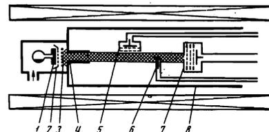
FIG. 1. Schematic illustration of the apparatus: 1—tungsten emitter, 2—electrode, 3—discharge cathode, 4—collimator, 5, 7—analyzer, 6—probe, 8—vacuum chamber.
